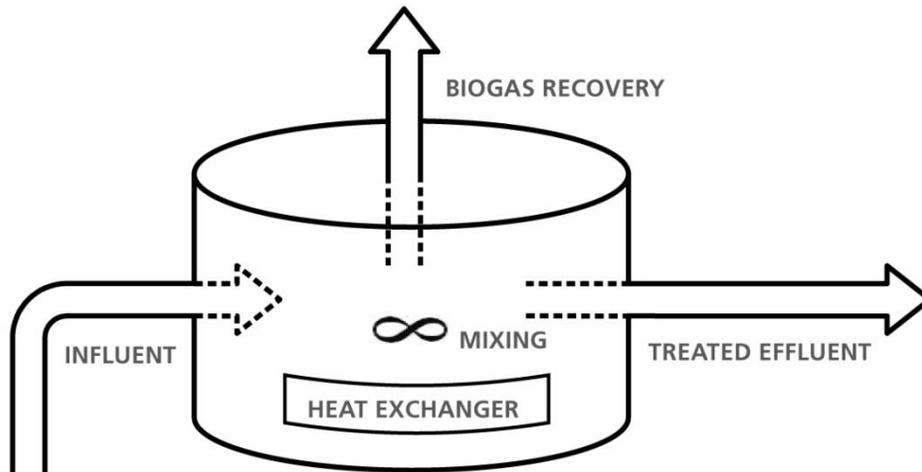
Figure 3 – Simplified complete mix digester schematic
