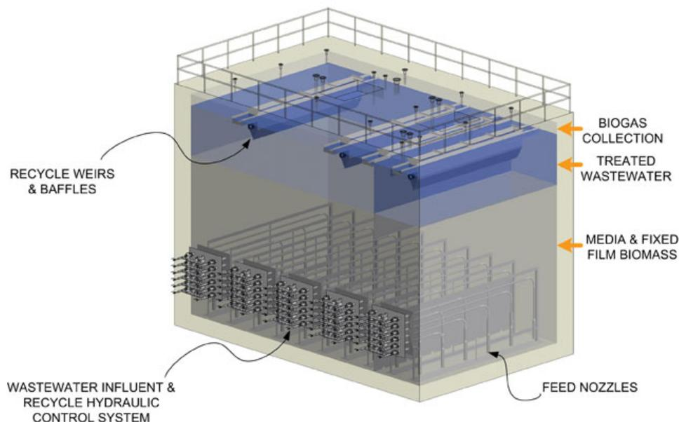
Figure 18 - MFT Digester Schematic. Graphic courtesy of Ecolab.
