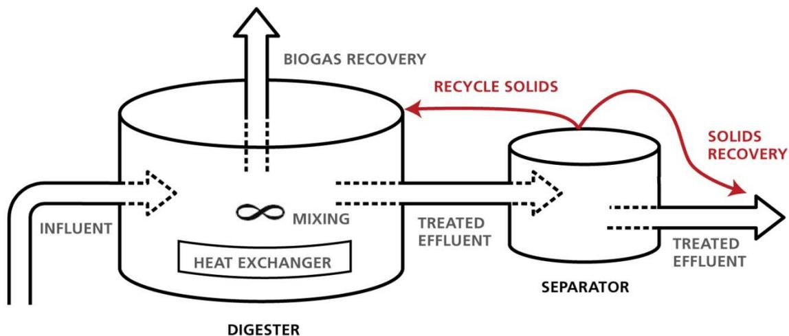
Figure 4 - Simplified anaerobic contact process schematic
