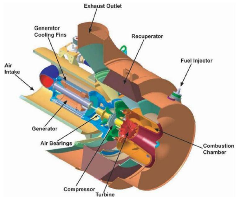
Figure 2. Microturbine illustration.
