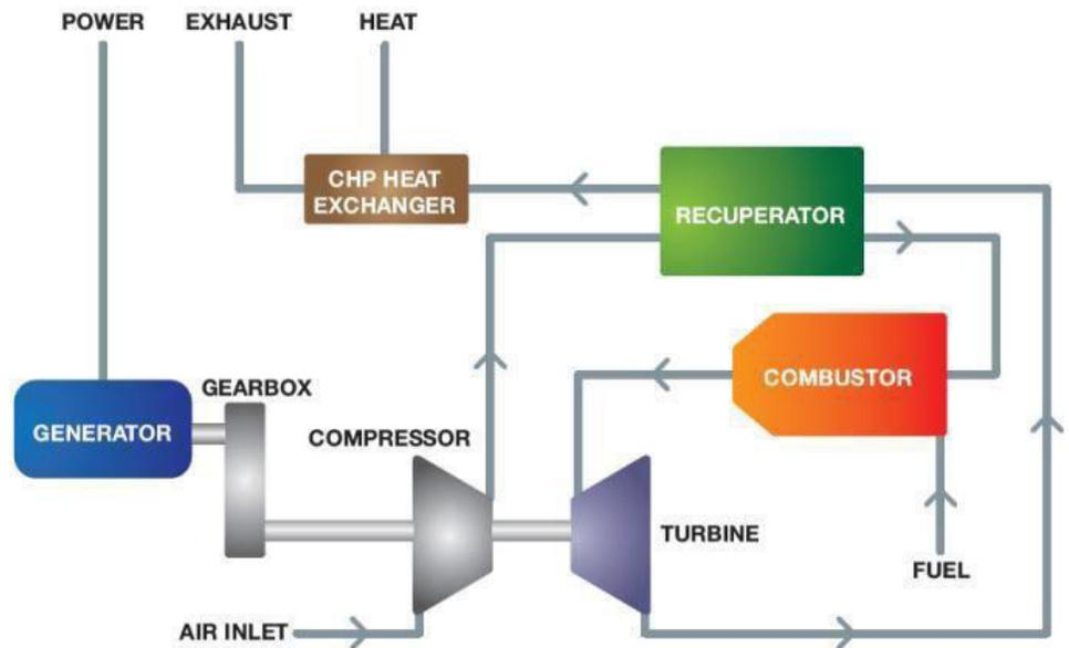
Figure 1. Microturbine configuration for CHP.
