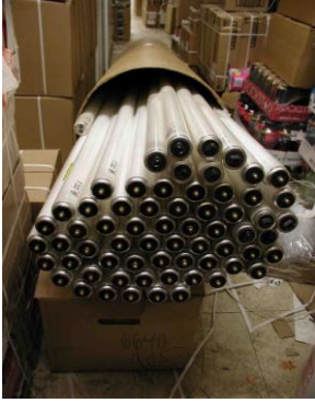
8ft, T-12 lamps prepared for recycling.
