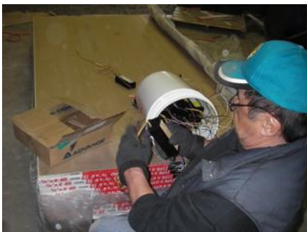
Double checking ballasts for PCBs
