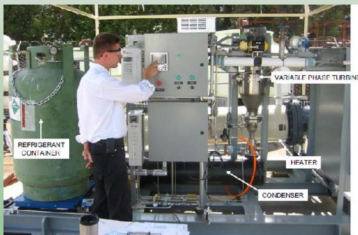
Figure 12. Variable Phase Turbine operating in pilot plant.
