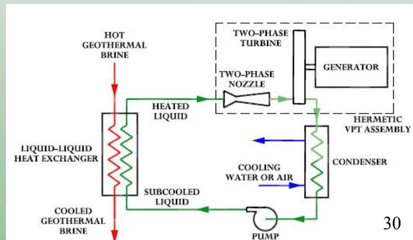
Figure 15. Variable Phase cycle process flow diagram.
