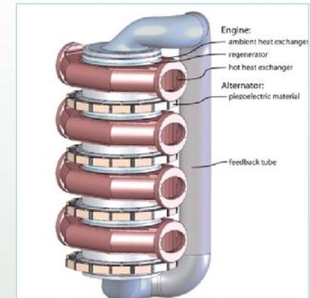
Figure 1. Thermocoustic piezoelectric generator, consisting of four thermocoustic Stirling engines driving four piezoelectric alternators.
