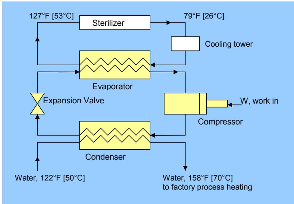
**Figure 17 - Example Heat Pump Application in a Dairy**
