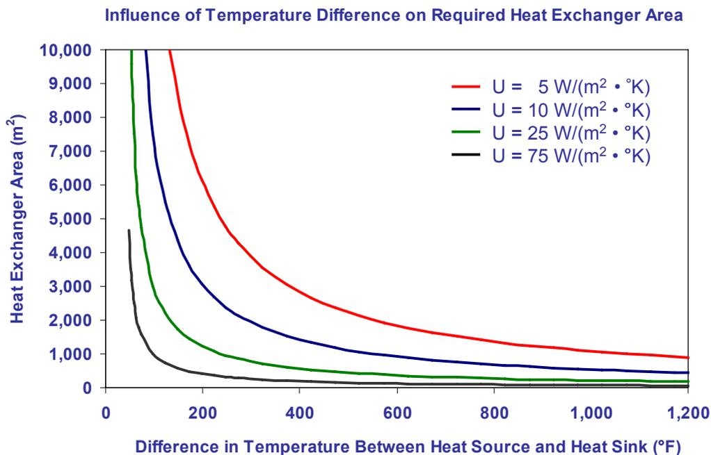
**Figure 1 - The Influence of Source and Sink Temperature (ΔT) on Required Heat Exchanger Area**
