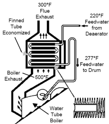
**Figure 10 - Finned Tube Exchanger / - Boiler Economizer** (Source: PG&E 2007) -
