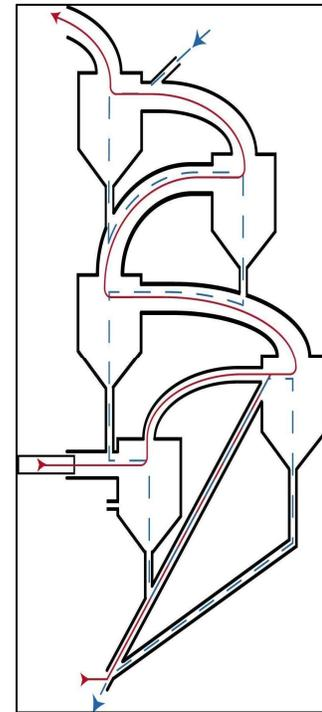
**Figure 21 - Cement - Kiln Preheater**
