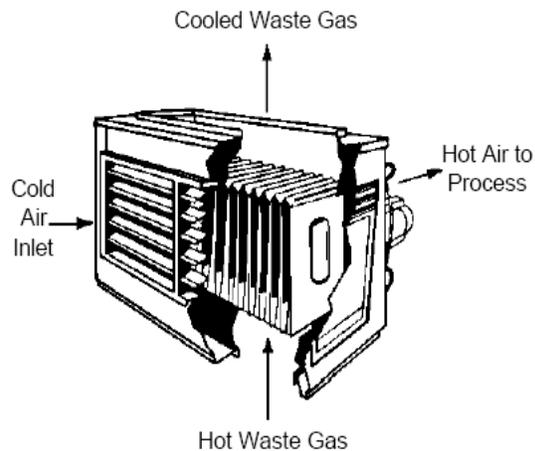
**Figure 8 - Passive Gas to Gas Air Preheater**
