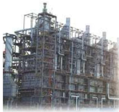
**Figure 28 - Ethylene Furnace**
